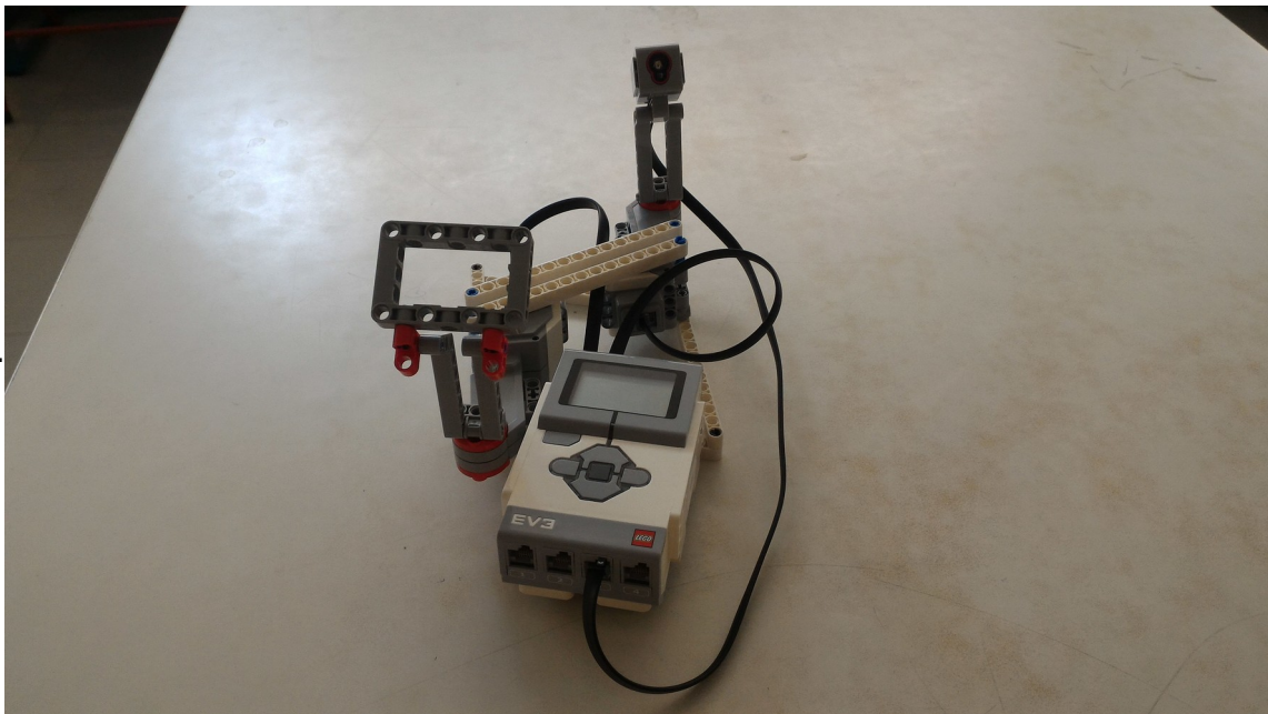
Image 2, The panel base can rotate in two axis. Vertical axis rotates automatically using the motor and Horizontal axis may rotate manually so that different panels can be attached
